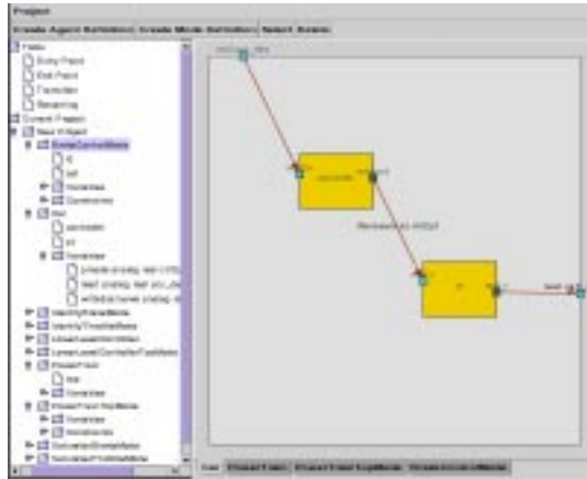
Fig. 8. The visual input tool of CHARON: The agent car is defined as the composition of two other agents. The arrows depict variable renamings.
